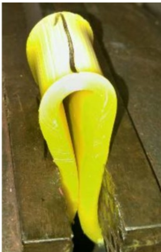
Figure 4: Image of Bend-Back Specimen Showing Inner Surface
