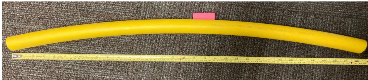
Figure 1: Sample of Exhumed Conduit
